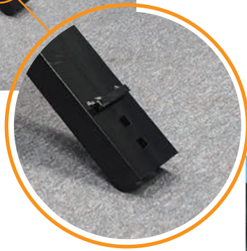
Welded Notch resting on the end rail
