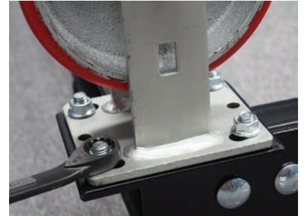
Attaching casters to the frame
